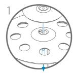
Pass the splash cable through the hole and pull it down.
